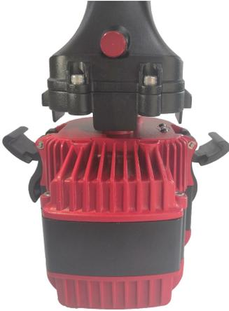
3. Push the hull cleaner electric brush down until it clicks into place, then close the clips on either side of the battery to lock it in place. The clips hold the battery pack in position and prevent it from detaching.
