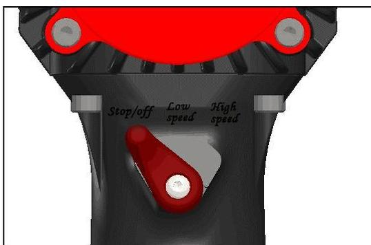
1. To turn the brush motor ON move the red switch at the back of the tool unit to **middle right** for low speed.
