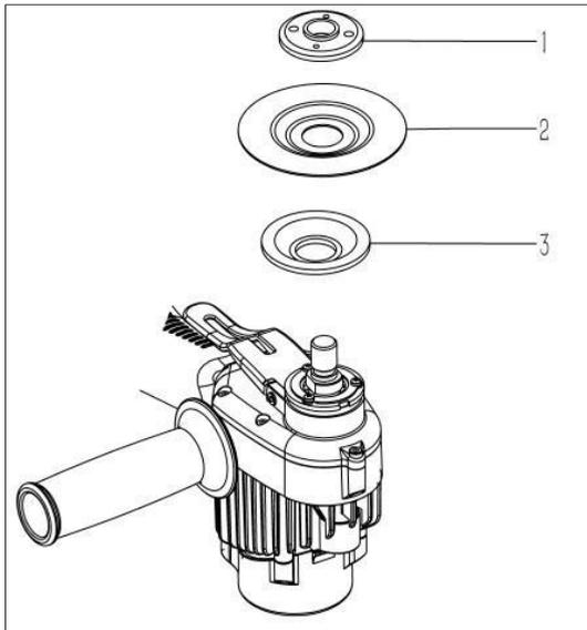
3. Position the disc (2) on top of the rubber pad.
