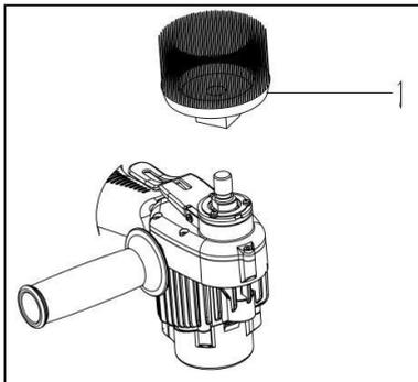
4. To remove the brush, press the shaft lock firmly to prevent the spindle from turning, then use the lock nut wrench to loosen the brush.
