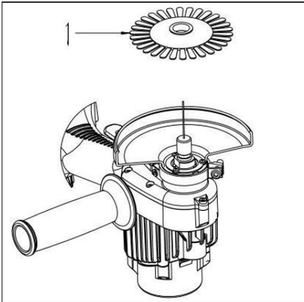
3. To remove the brush, press the shaft lock firmly to prevent the spindle from turning, then use the lock nut wrench to loosen the brush.
