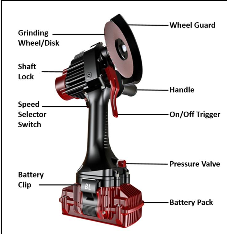
The On/Off trigger is a dead-man's switch, and provides important safety functionality. When you release the On/Off trigger, it immediately cuts off power to the motor and stops the angle grinder. You can only restart the angle grinder by moving the speed selector switch to the Off (0) position before pressing the On/Off trigger again, as described in *Switching the Angle Grinder On or Off*, page 24.
