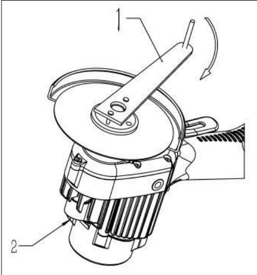
5. To remove the wheel or disc, press the shaft lock firmly to prevent the spindle from turning, then use the lock nut wrench to remove the lock nut from the spindle, freeing the wheel and flange.
