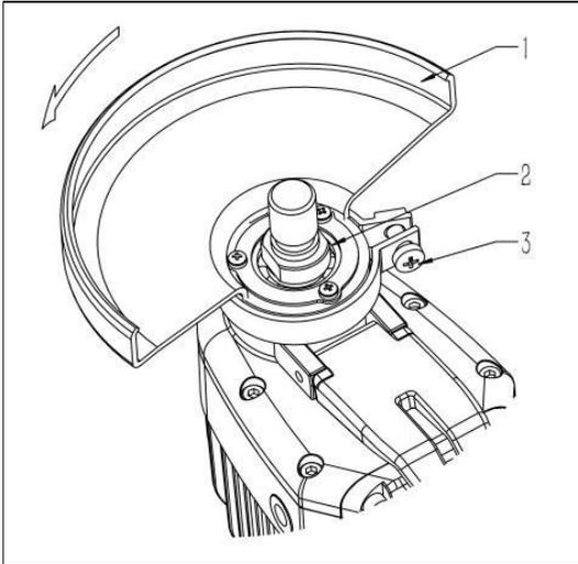
3. Rotate the wheel guard 180 degrees, and tighten the screw (3) securely.
