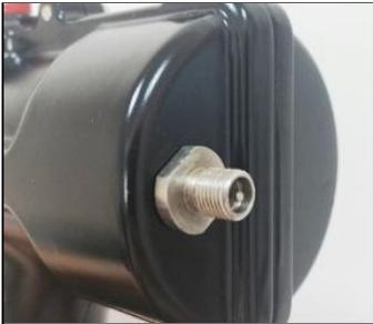
2. Attach a pump, such as the hand pump supplied with the impact driver, to the valve.
