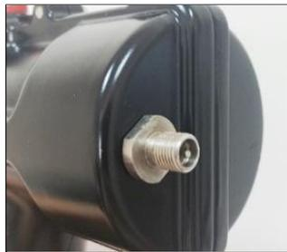
2. Attach a pump, such as the hand pump supplied with the impact wrench, to the valve.
